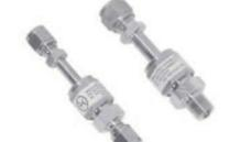
The HOKE Gyrolok Dielectric Tube Fittings are for use in applications where electrical current flowing through a pipe or tube line must be interrupted to protect vital instrumentation and metering equipment.
